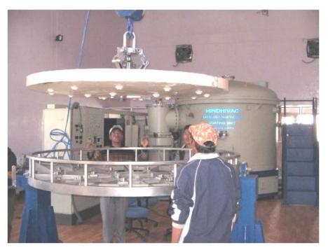
Fig 3a: Integration of dummy mirror with tilting mechanism
