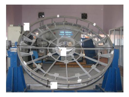
Fig 7: Tilting Fixture & Rotation Mechanism
