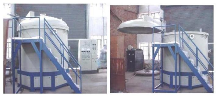
Fig 4: 2.5M diameter vacuum coating plant.
