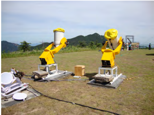
Figure 1.1: The two 40-cm telescopes at the Indian Camp at Anji, China which imaged the solar corona in the green and red emission lines during the total solar eclipse of July 22, 2009.
