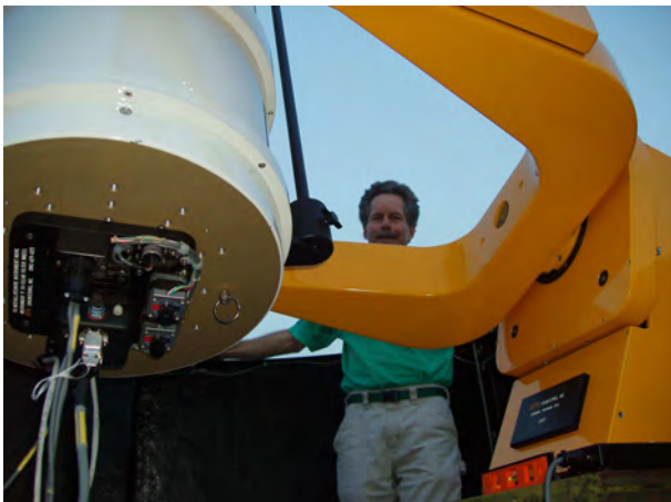
Figure 2.10: The 40cm DIMM telescope mounted atop the tower at VBO. The DIMM instrument is mounted at the cassegrain focus which is within the telescope tube. Only the CCD camera and some controls are seen outside. Mark Kelley of DFM is seen in the picture.
