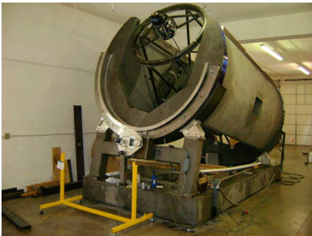
Figure 2.13: Assembled structure of the 1.3m telescope viewed from the N-W side. The RA axis drive assembly is seen on the face of the horseshoe. The north side horseshoe is on two hydrostatic bearing pads. The top ring of the telescope truss assembly and the 5-axis positioner for the secondary mirror are also seen.
