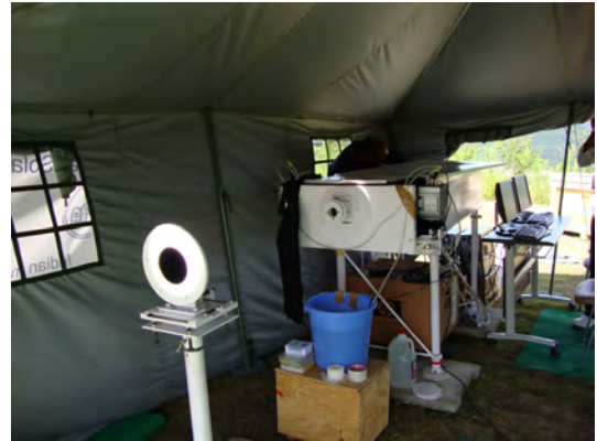
Figure 1.2: The spectrograph at the Indian Camp at Anji, China which was used to take spectra of the solar corona in the green and red emission lines during the total solar eclipse of July 22, 2009.
