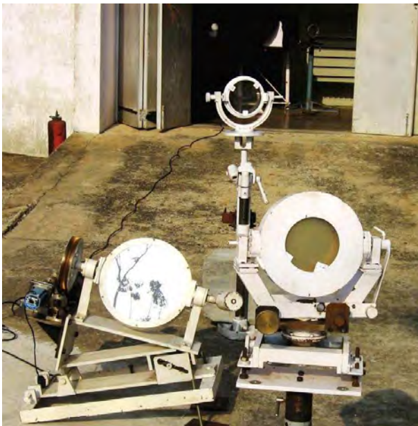
Figure 2.6: Optical light path arrangement and tracking of the solar image to the spectrograph during the total solar eclipse experiment.
