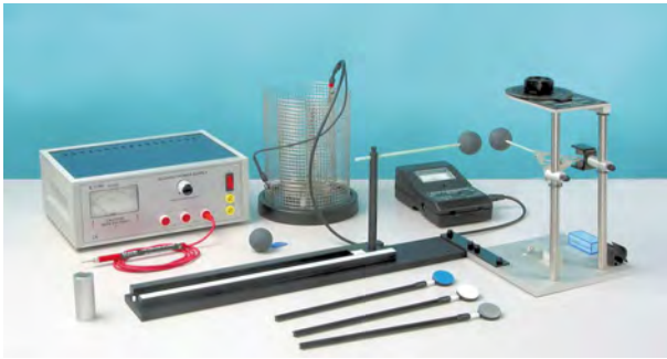
Experimental setup for verification of Coulomb's law of electrostatics force.
