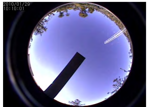
Figure 2.26: A sample all-sky frame at Devasthal obtained on 29 January 2010. The tree line and the 15 m micro thermal tower are seen in the frame. The dark strip blocks the sun to provide a fish-eye view of the sky.
