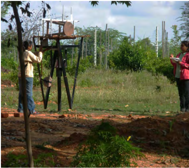
Students of Pune University measuring the radiation pattern of the antenna they fabricated at the Gauribidanur observatory.
