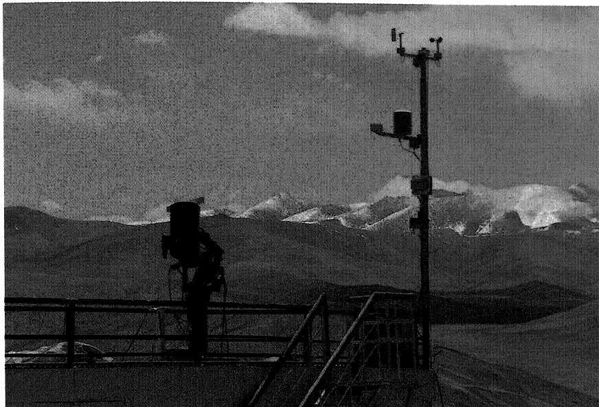
Figure 22: SDIMM and SHABAR equipment with a weather station at Hanle.
