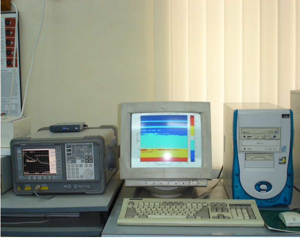
Figure 24: Gauribidanur Radio Array Solar Spectrograph (GRASS). The Agilent spectrum analyzer along with control and data acquisition PC are shown.
