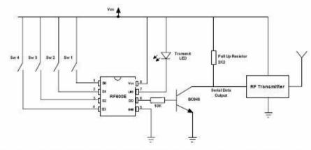
Not that a circuit constructed using AM radio modules does not need to have transistor BC848, resistor 10K or 2k2 Pull up resistor fitted.
