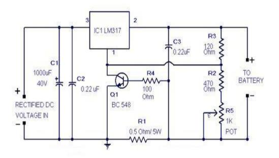
Fig 3 : Simple Lead Acid Battery Charger using LM317.
