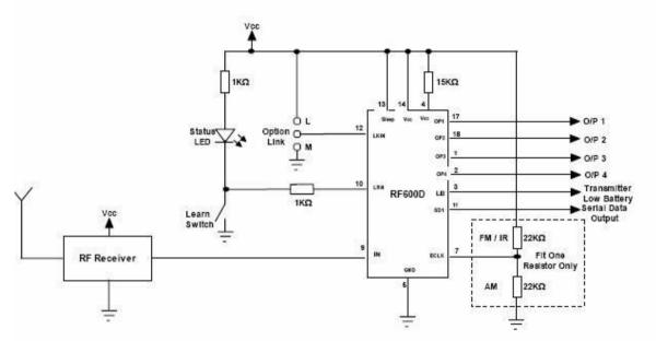
This circuit provides a complete decoding solution capable of learning up to 7 unique encoders
