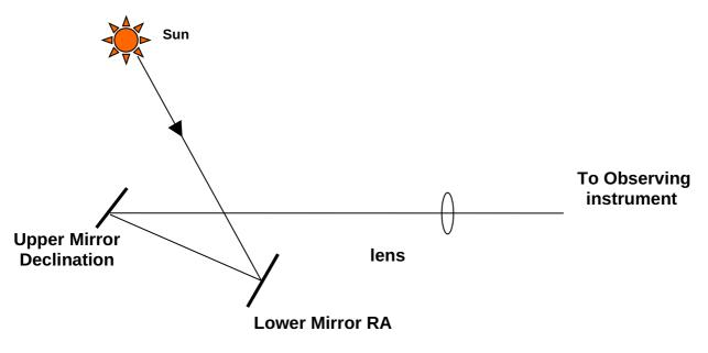
Figure – 1 Coelostat mirror arrangement
