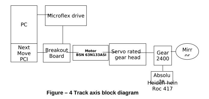
The track axis block diagram is shown above. The two guide axes also has the same components
