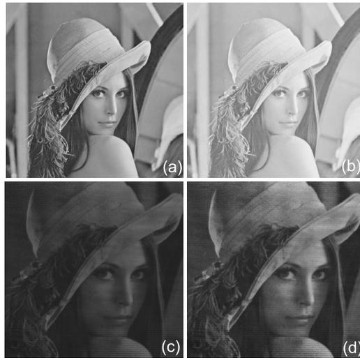
**Figure 5.** (a) Original *Lena* image, (b) transformed image, (c) SLM output for the original image and (d) SLM output for the transformed image captured on CCD.
