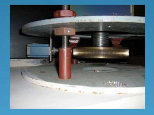
Stepper Motor KML 063 being used for positioning the Grating at 24" Solar Tower Tunnel Telescope, Kodaikanal
