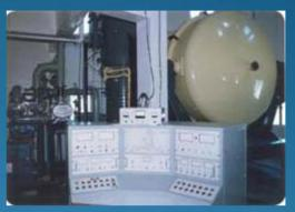
2.8M Vacuum Coating Plant, VBO being used for coating 2.34M primary mirror of the VBT
