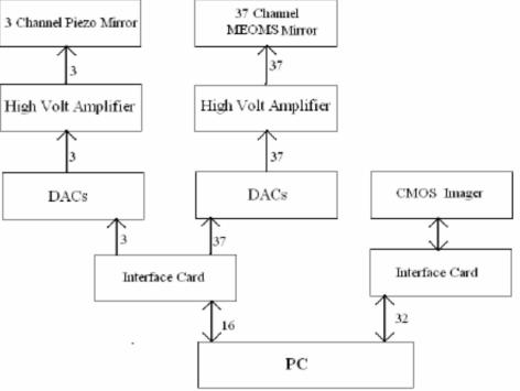
Schematic of electronic control of tip-tilt mirror, deformable mirror and wave-front sensor camera
