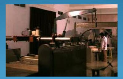
The 50 inch polishing machine which was indigenously built at IIA and used for fabricating 50 inch f/1.45 Hindle's sphere which was used as Hindle sphere for 2.34 M Telescope secondary mirror testingf - can be seen at the Photonics lab.
