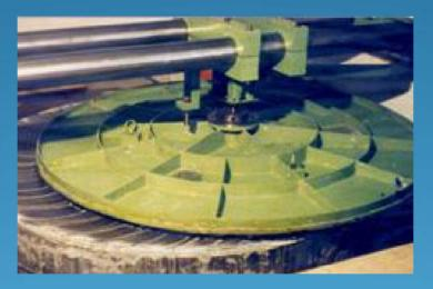
Some of the pictures related to the fabrication of 2.34M primary mirror of the Vainu Bappu Telescope.
