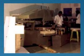
The picture shows 30 inch & 18 inch polishing machines. The primary mirror of the 30 inch telescope optics were fabricated using these machines during 1980s.
