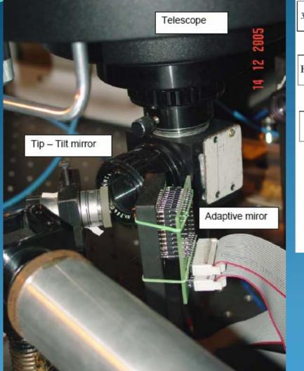
A view of the experimental setup showing tip-tilt mirror and adaptive mirror
