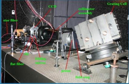
This instrument was commissioned in 2003 and since then it has been used for optical astronomy. This instrument works in Litrow configuration and single collimator unit is used and same is used as camera for focusing spectra.
