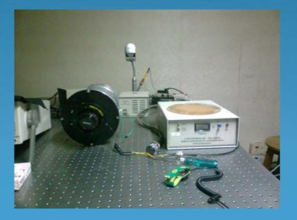
Lab setup for acquiring an image using CCD DEWAR.
