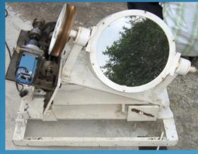
KML 063 & MD 808 being used in the Coelostat for tracking Solar image, during Total Solar Eclipse expedition.
