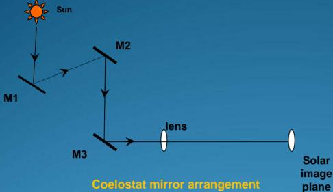
The first mirror M1 tracks the sun and second mirror guides the image in the image plane. There are three axes to be controlled one track axis and two Guide axes RA and DEC. Motor speed for track axis at 7.5 arc sec/sec = 0.9 RPM, Guide axis motor speed at 0.25 degrees/sec = 1000 rpm
