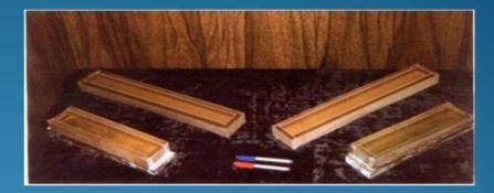
Two sets of Synchrotron Radiation Beam Line Optics (SRBL) for Bhaba Atomic Research Center funded by BRNS was fabricated and delivered. The optics consists of spheroidal and plane mirrors.
