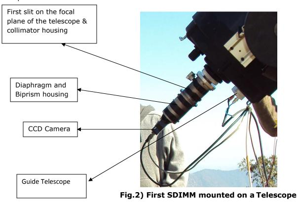
The limb motion is recorded on the CCD and 150 to 200 frames are grabbed in a 10 sec period. Exposure time for each frame given is around 1ms. The data of limb position on the two slit is used to derive the r0 value<sup>(5)</sup>. This is accomplished by computing the variance of the limb differences over the 10 seconds of data using the following expression for variance:
