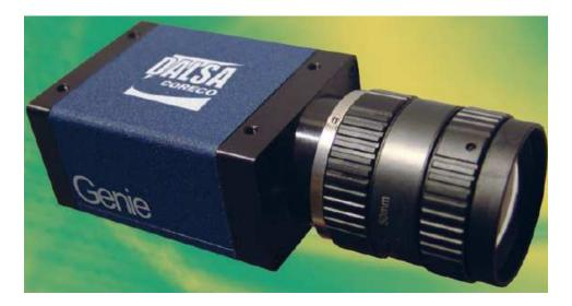
The Genie M640 with a resolution of 640 x 480 CCD has been used. Operating at 60 frames per second at full resolution, the Genie M640 takes advantage of gigabit Ethernet technology for transmitting data and direct link from the camera to a PC.All Genie cameras are supported by DALSA's Sapera<sup>™</sup> LT software libraries featuring CamExpert for simplified camera set-up and configuration.
