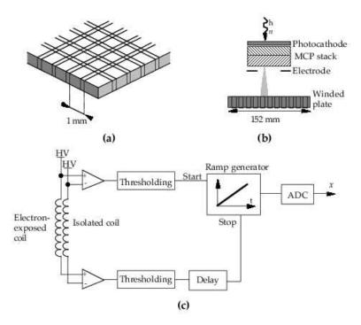
Figure 12: (a) Sobottka & Williams' delay-line anode, (b) camera using this anode, and (c) Readout electronics of this camera.
