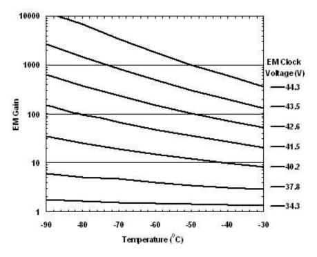
Figure 15: Temperature vs. gain.
