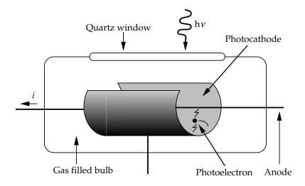
Figure 2: Principle of a Geiger gas detector.
