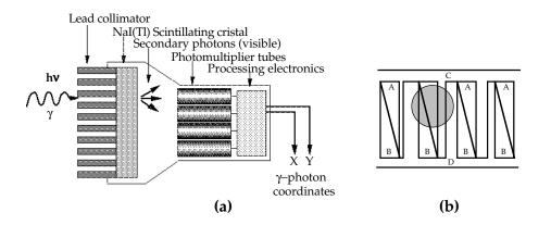
Figure 9: (a) Anger gamma camera and (b) wedge-and-strip anode. The grey disk corresponds to the cloud of electrons that is spread onto a local area of the anode.
