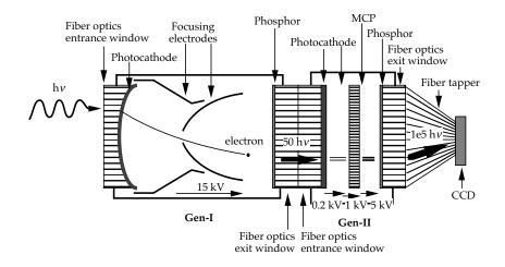
Figure 6: Classical design of an intensified-CCD photon-counting camera. The represented Gen-II intensifier features proximity focusing (which reduces the image distortion).
