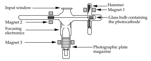
Figure 4: A Lallemand tube used for astronomy. The ring magnet 1 is used to move the hammer and break the glass bulb containing the photocathode. The ring magnet 2 is used to bring the photocathode behind the input window. The ring magnet 3 is used to change the photographic plate.
