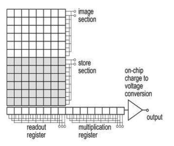
Figure 14: Structure of a typical L3CCD sensor.
