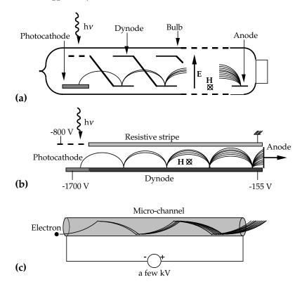
Figure 3: (a) MS-10 photomultiplier, (b) continuous dynode photomultiplier, and (c) micro-channel.
