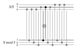
Figure 11: Principle of coordinate encoding of a MAMA camera (imaginary case with N = 3). The grey zone represents the impact of the cloud of photons on the anode. The activated electrodes are represented in black.
