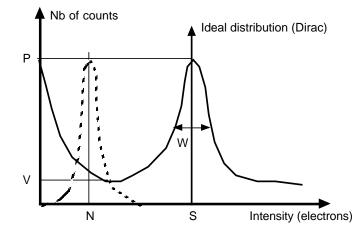
Figure 1: Example of a usual PHD. The dashed curve is the noise statistics of the detector readout. PV = P/V and NFWHM = W/S. The usual PHD is a Dirac's peak.
