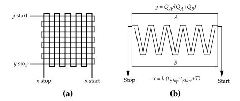
Figure 13: (a) Friedman's serpentine delay-line anode and (b) Lampton's hybrid wedge-and-strip + delay-line anode.
