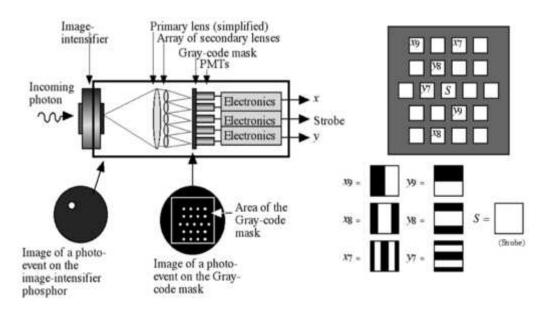
Figure 7: The PAPA camera. Coding mask elements are shown on the right.
