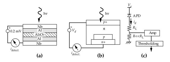
Figure 16: (a) Principles of an STJ, and (b) of an APD, (c) Passive quenching of an APD.
