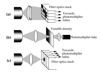
Figure 5: Three systems for measuring the photon position by Iredale et al. [35].
