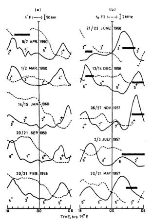
Fig. 1—Typical examples of the nocturnal variation of h'F and  $f_0F2$  at the equatorial station, Kodaikanal, showing the presence of an increase in F-region height in the post-midnight period: (a) without the occurrence of spread-F and (b) with the occurrence of spread-F (The black patches on the plots indicate the presence of spread-F. Values of the 3-hourly planetary geomagnetic index,  $K_{pp}$  are also shown)
