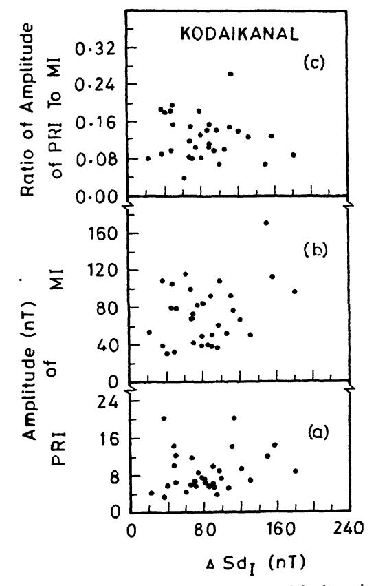
Figure 1. Variation with the equatorial electrojet strength ( $\Delta$  SdI) of (a) magnitude of preliminary reverse impulse (PRI) (b) magnitude of main impulse (MI) and (c) ratio of the magnitude of PRI to MI for SC SC(-+) events at Kodaikanal.
