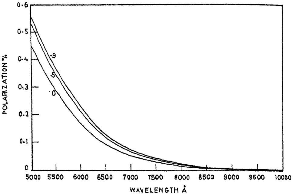
Fig.4 Polarization versus wavelength for  $m_2/m_1 = 0, .5, .9$  (mentioned on the graph)
