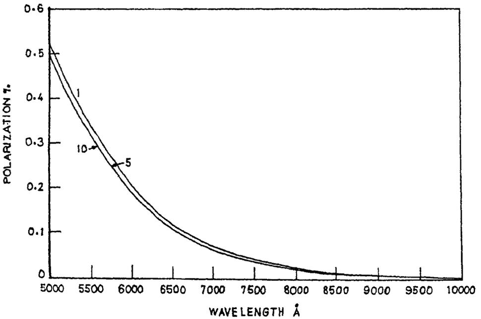
Fig.5. Polarization versus wavelength for  $x = 1, 5, 10$  (mentioned on the graph)
