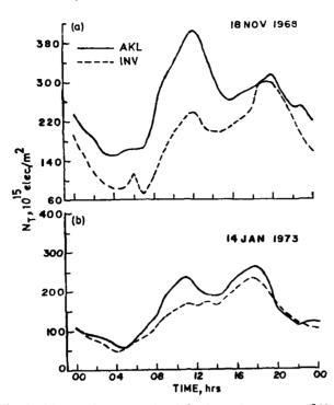
Fig. 4—(a) A typical example of the diurnal variation of  $N_T$ at Auckland and Invercargill showing opposite nature in the structure of the bite-out pattern at the two stations; (b) A typical example of the diurnal variation of  $N_T$  at Auckland and Invercargill showing the conspicuous absence of the bite-out at one of the two stations
