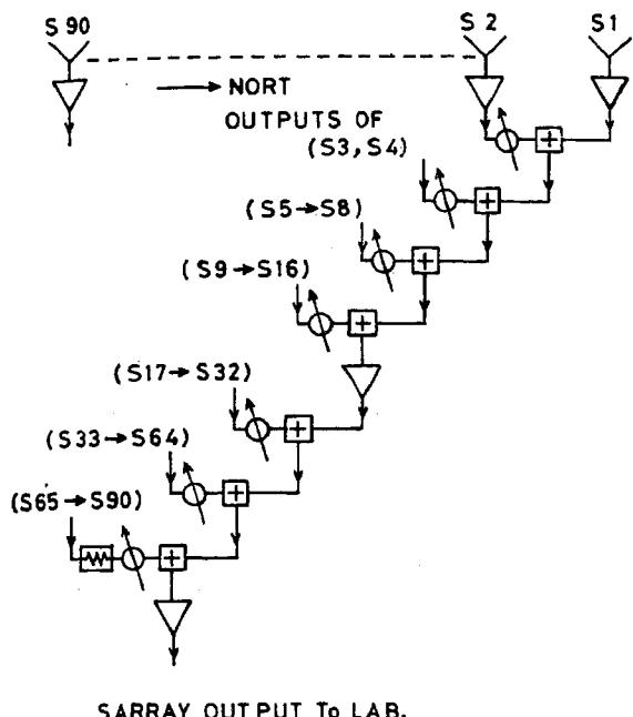
Fig. 6—Configuration of the South array
