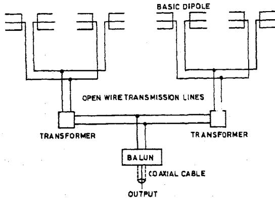
Fig. 2—A basic array element consisting of four dipoles connected in a branched feeder system
