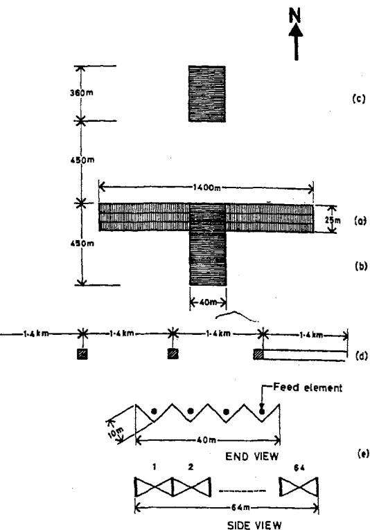
Fig. 3—Lay-out and dimensions of various antenna arrays at Gauribidanur (a) East-West array: 4 rows in N-S direction, 160 dipoles in each row; (b) South array: 90 rows in N-S direction, 4 dipoles in each row; (c) North array: 64 rows in N-S direction, 1 Yagi in each row; (d) Compound grating interferometer: E-W array and 4 grating units. Each grating unit consists of 8 Yagis; (e) Broadband array: 64 conical dipoles arranged in a matrix of  $4 \times 16$  along E-W and N-S directions respectively
