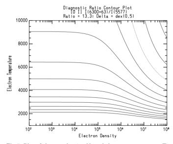
Fig. 7. Plot of electron density  $N_{\rm e}$  and electron temperature  $T_{\rm e}$ . The dotted line is the contour for the observed ratio (13.3) of [O]I lines 5577 Å, 6300 Å and 6363 Å. Each contour in the plot is for a change in the flux ratio of 0.5
