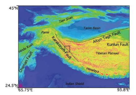
**Figure 1.** Topographic map of central Asia, based on satellite digital elevation data, showing topographic expression of tectonic features, including major active faults. The region of our study, shown in more detail in Figure 2, is outlined.
