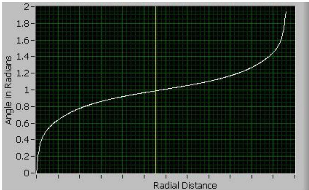
**Figure 7.16** The radial profile after the  $2\pi$  ambiguity removed
