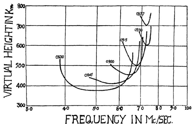
Fig. (5).—Ordinary component of h'f trace showing rapid upward drift of the pre-eclipse F<sub>2</sub> layer.
