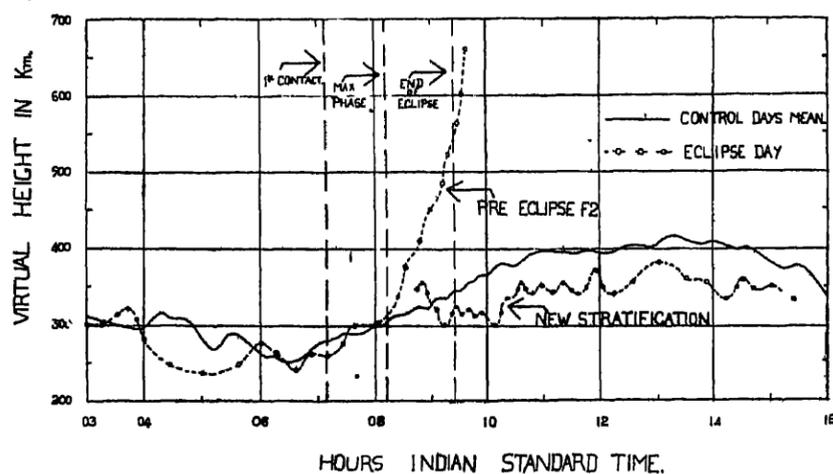
Fig. (6).—Virtual heights of F<sub>2</sub> layer on eclipse day and mean control day.
