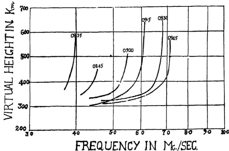
Fig. (4).—Ordinary component of the h'f curve showing development of the new F region,
