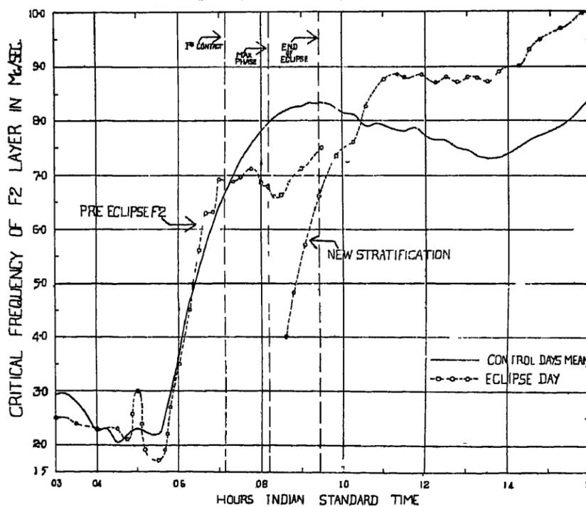
Fig. (1).—F<sub>2</sub> Layer critical frequencies on eclipse day and mean control day.
