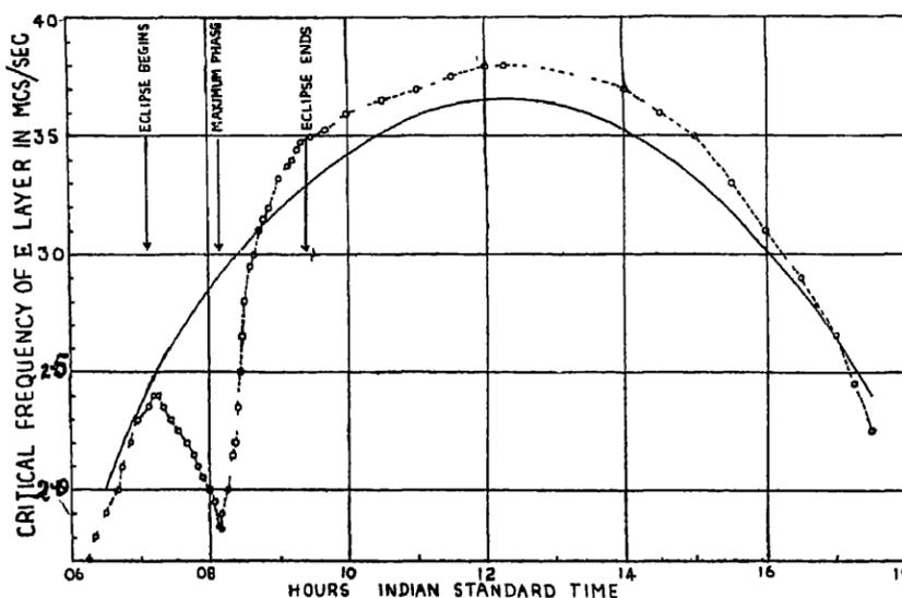
Fig. (1).—Variation of critical frequency of the E layer during the eclipse.— median of control period values. o-o-o-o values observed on eclipse day.
