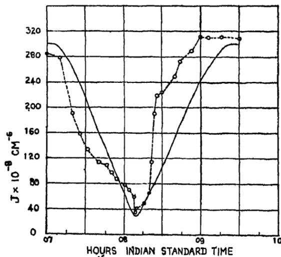
Fig. (2).—Changes in the E layer ionising radiation during the course of the eclipse. — calculated assuming uniformly radiating solar disc. o-o-o-o observed values.
