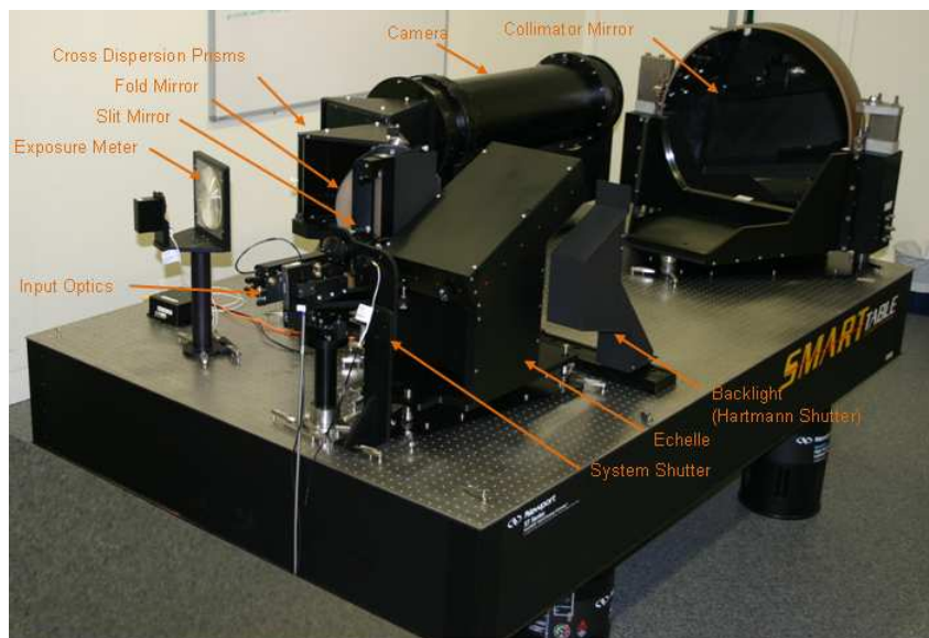
Figure 2.9: Hanle Echelle Spectrograph aligned and tested at the Kiwistar Optics Facility (Image credit : Callaghan Innovation)
