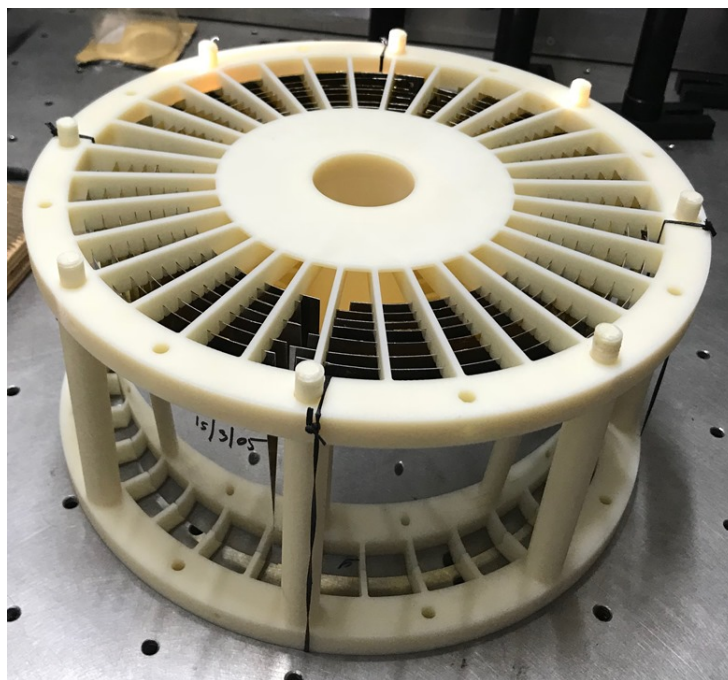
Figure 7.16: Photograph of the prototype X-ray concentrator developed using SXT spare mirrors. The mechanical structure in 3-d printed using URSC facility.
