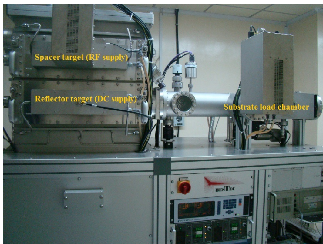
Figure 3.5: Picture of magnetron sputtering system at RRCAT which is used to fabricate all multilayer mirrors discussed in this thesis.
