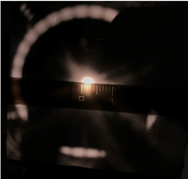
Figure 7.19: Photograph of the spot at the focal plane screen of the concentrator.
