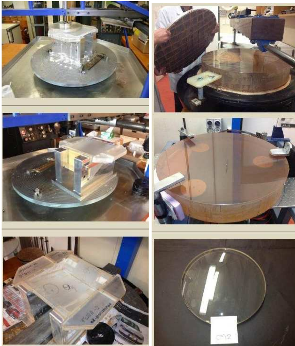
Figure 3.25: The fabrication process of the prism is illustrated in the left column and the right column shows the polishing process for the collimator mirror and one of the camera lens after polishing.
