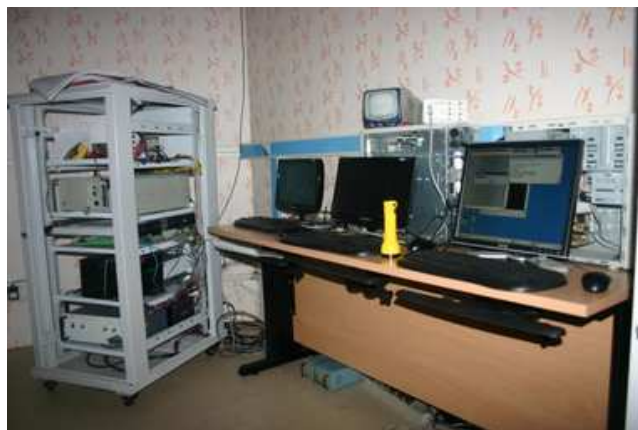
Figure 3.16: A view of the console rack in the 75 cm telescope control room.
