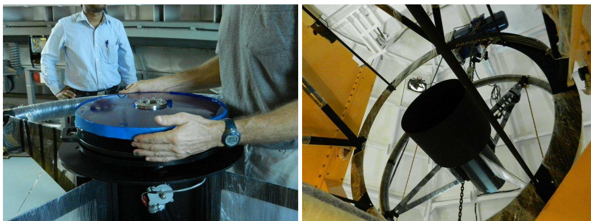
Figure 3.13: (left) Secondary mirror fixed on the 5 axis mount within the top ring. (right) Top ring being mounted on truss assembly – 9th March.
