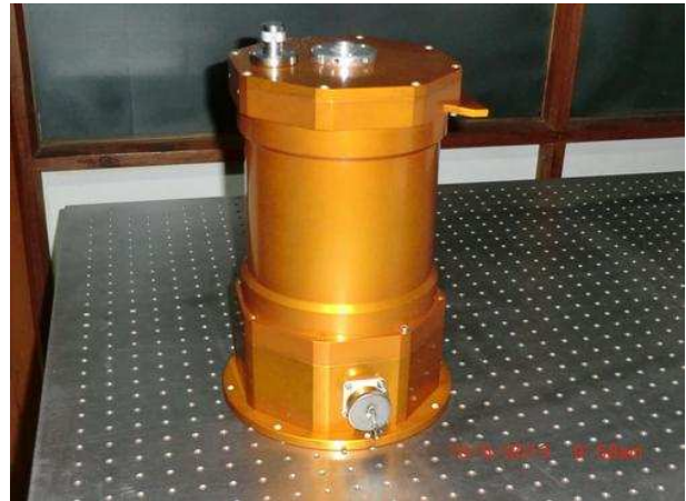
Figure 1.28: A view of the dewar for 2K×4K camera.
