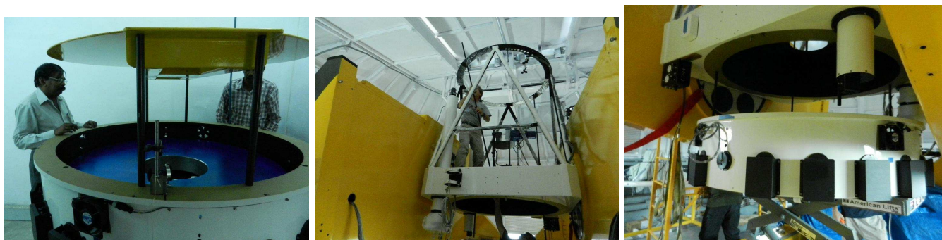
Figure 3.12: (left) Mirror mounted in cell, before lifting up through the pier. The blue coating is a peelable protective layer. The cover top is for protection during the lift operation. (middle) The upper truss structure in place. The black invar rods serve as reference for the spacing of the primary and secondary mirrors. (right) Mirror cell being raised using the hydraulic trolley for mounting on the centre section – 8th March.
