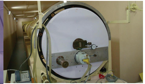
Figure 3. Sixty feet Littrow type spectrograph in the about 210 feet long tunnel of the Solar Tower Telescope.
