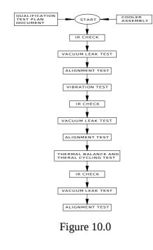
Different models will be fabricated to fully qualify any newly designed subsystem before using in the spacecraft. Similarly three models of INSAT 3D coolers are fabricated. They are structure model (STM), electrical thermal model (ETM) and flight model (FM).The test sequence is shown in figure 10.0
