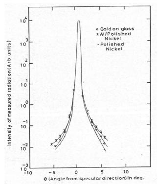
The measurement of reflected light distribution was done using He-Ne laser. Figure 8.2 shows the curves for polished nickel, and a gold deposited glass slide. As can be seen from the above, the reflected diffused radiation lies in a cone of  $5^{0}$ about about the specular direction. Also the reflected energy distribution from polished samples compares extremely well with that from the gold on glass sample thereby demonstrating excellent finish
