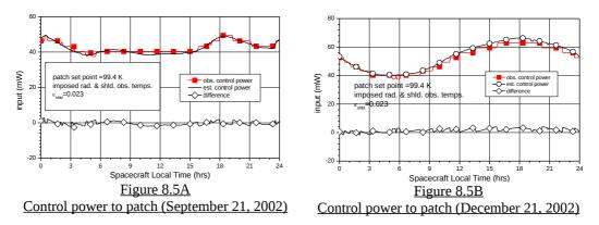
The flight performance of the VHRR radiant cooler has been satisfactory till date. Analysis of flight data indicates that a patch temperature less than 105K has been achieved during the first summer solstice the spacecraft experienced after the launch. The patch temperature at the first equinox has been less than 89K. Also for the first two winter solstices, the patch temperature remained below 89K.
