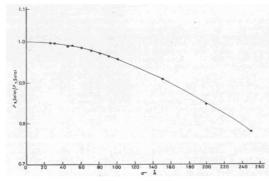
Figure 7.0 Variation of  $\rho_s$  solar /  $\rho_T$  solar for small values of surface roughness
