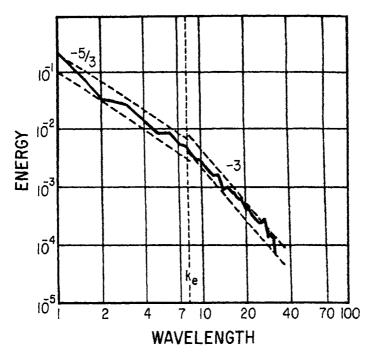
Fig. 3. An omnidirectional energy of two-dimensional Navier-Stokes turbulence obtained numerically (Lilly 1969). The initial spectrum dominated by the source spectrum at the source wave  $K_e$ , is shown to relax to the inertial range spectra for enstrophy at  $K > K_e$  and energy at  $K < K_e$ .
