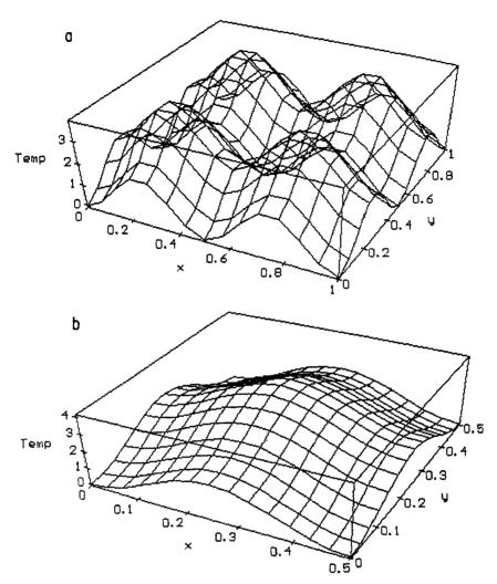
Fig. 2. Spatial distribution of temperature calculated from Eq. (23) in a region (x/a, y/a) = (0,0) to (1,1) plot (a) and (0,0) to (0.5,0.5) plot (b).
