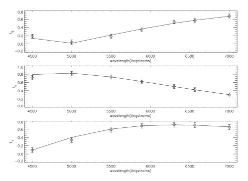
Figure 2. Plots of polarimetric efficiency of Stokes Q, U and V parameters as a function of wavelength. The solid curves are theoretical values whereas the diamond symbols correspond to the measured values. The error bars shown in these plots are ten times the obtained noise rms values.
