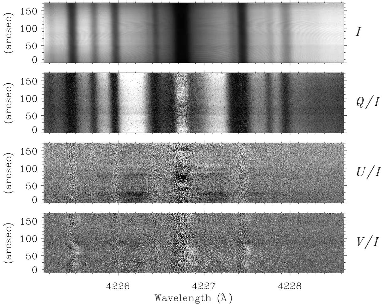
Fig. 1.— CCD images of the Stokes parameters recorded with the spectrograph slit parallel to the limb ( $5''$  inside the limb). Note the depolarization signatures in the  $Q/I$  wings in the  $55''$  -  $75''$  spatial interval. Corresponding  $U/I$  wing signatures are seen at the same wavelength positions, but at a different spatial location, for example in the  $20''$  -  $30''$  interval.
