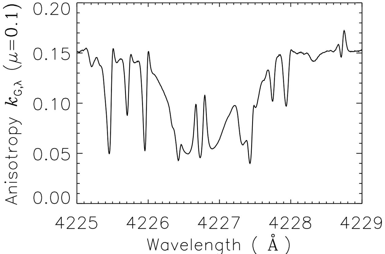
Fig. 3.— Plot of the geometric depolarization or anisotropy factor  $k_{G,\lambda}(\mu)$  as a function of  $\lambda$  for disk position  $\mu = 0.1$ .
