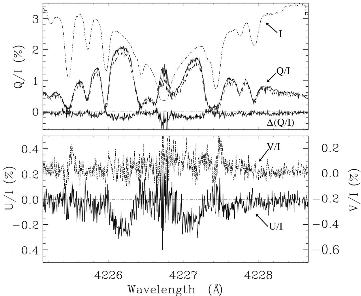
Fig. 2.— Stokes  $I$ ,  $Q/I$ ,  $U/I$ ,  $V/I$  profiles extracted from Fig. 1. The heliocentric angle corresponds to  $\mu = 0.1$ . Note the depolarization in the  $Q/I$  wings and the  $U/I$  signatures at the corresponding wavelength positions. In the present paper we refer to them together as the “( $Q/I, U/I$ ) wing signatures”.
