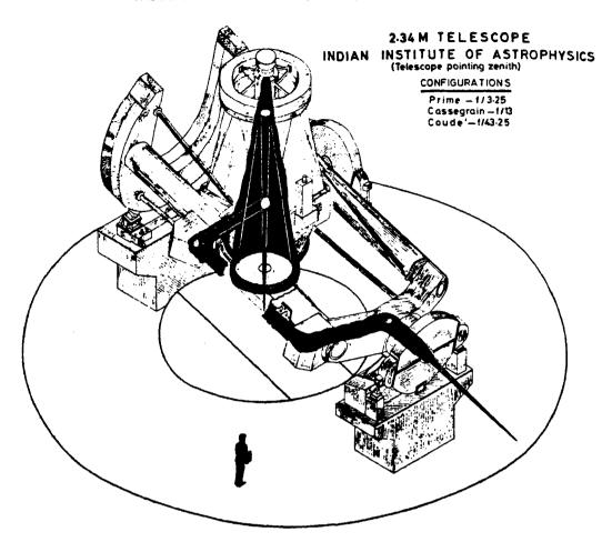
Fig. 6—Sketch of the proposed optical system
