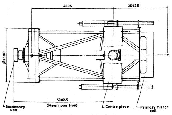
Fig. 2—Serrurier truss of 234 cm telescope
