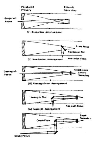
Fig. 1-Variations in reflector telescopes
