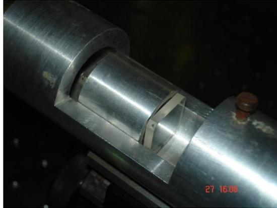
**Fig.7.9 A close up view of the mounting of the two crosses Babinet compensators in a cell**
