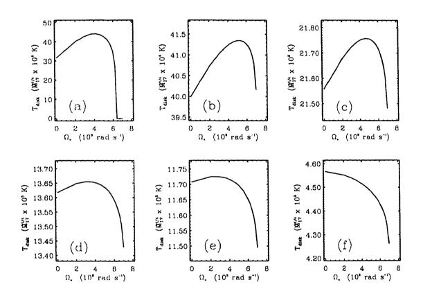
Figure 3.9: Plots of  $T_{\text{disk}}$  vs.  $\Omega_*$  at various chosen radial distances: (a) r = 13 km, (b) r = 35 km, (c) r = 100 km, (d) r = 200 km, (e) r = 250 km and (f) r = 1000 km. These are for EOS model (B), an assumed gravitational mass value of 1.4  $M_{\odot}$ , and the same values of  $\eta$ ,  $\beta$ , h/r and n as in Fig. 3.8 are used.
