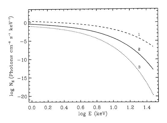
Figure 5.2: Accretion rate dependence: general relativistic spectra including light-bending effects from accretion disk around a neutron star of mass-shed limit configuration ( $\Omega_* = 7001 \text{ rad/s}$ ). Curve (1) corresponds to  $\dot{M} = 10^{18}$  g/sec, curve (2) to  $\dot{M} = 10^{17}$  g/sec and curve (3) to  $\dot{M} = 2 \times 10^{16}$  g/sec. The values of all the other parameters are as in Fig. 5.1.
