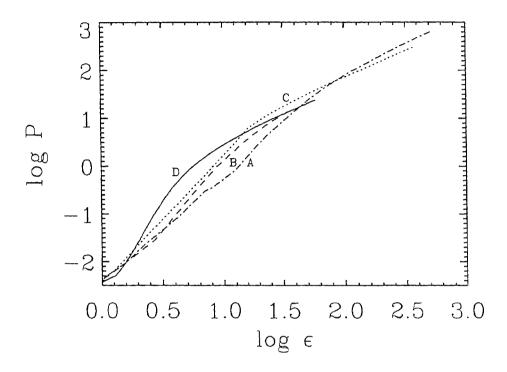
Figure 2.1: Logarithmic plot of pressure vs. matter density for the EOS models used here. The density and pressure are in units of  $1.0 \times 10^{14}$  g cm<sup>-3</sup> and  $(1.0 \times 10^{14})$   $c^2$  cgs respectively.
