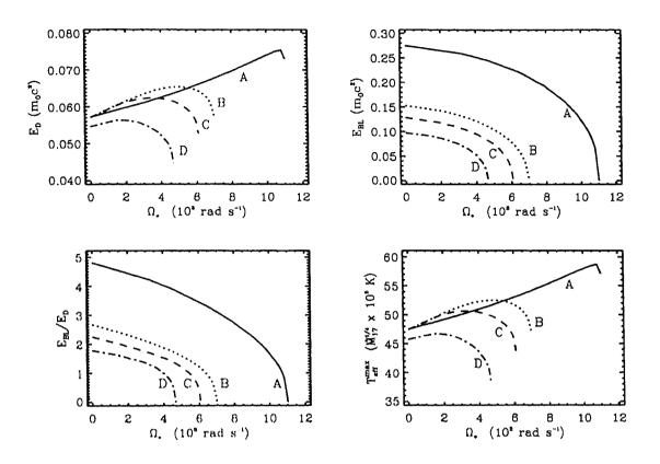
Figure 3.5: The variations of the  $E_{\rm D}$ ,  $E_{\rm BL}$ ,  $E_{\rm BL}/E_{\rm D}$  and  $T_{\rm eff}^{\rm max}$ , with  $\Omega_*$  for a chosen neutron star mass value of 1.4  $M_{\odot}$  for the four EOS models. The curves have the same significance as Fig. 3.3b.
