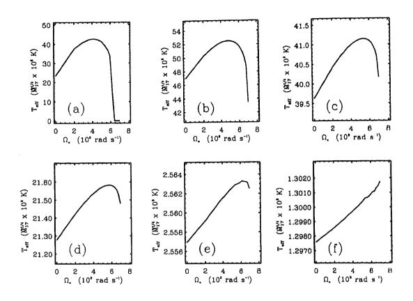
Figure 3.4: Plots of  $T_{\text{eff}}$  vs.  $\Omega_*$  for chosen constant radial distances for fixed neutron star mass  $M = 1.4 \ M_{\odot}$  and EOS model B. The plots correspond to (a)  $r = 13 \ \text{km}$ , (b)  $r = 18 \ \text{km}$ , (c)  $r = 35 \ \text{km}$ , (d)  $r = 100 \ \text{km}$ , (e)  $r = 2000 \ \text{km}$  and (f)  $r = 5000 \ \text{km}$ .
