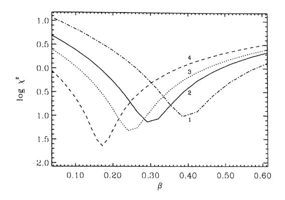
Figure 6.3: Variation of minimum  $\chi^2$  (i.e. minimized with respect to parameters  $E_a$  and  $S_o$ ) with parameter  $\beta$ . Curves marked 2, 3 and 4 correspond to the spectra shown in Fig. 3 for  $i = 0^{\circ}, 30^{\circ}$  and 60° respectively. Curve marked 1 is for the Newtonian spectra shown in Fig. 6.1.
