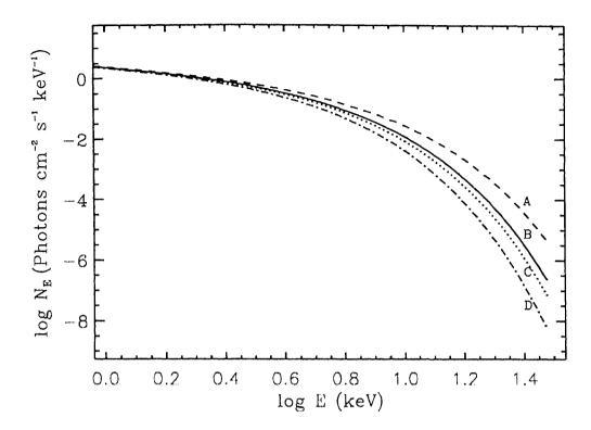
Figure 5.5: EOS model dependence: general relativistic spectra including light-bending effects from accretion disk around a neutron star of mass-shed configuration. EOS model (A) is for  $\Omega_* = 11026 \text{ rad/s}$ , model (B) is for  $\Omega_* = 7001 \text{ rad/s}$ , model (C) is for  $\Omega_* = 6085 \text{ rad/s}$  and model (D) is for  $\Omega_* = 4652 \text{ rad/s}$ . The values of all the other parameters are as in Fig. 5.1.
