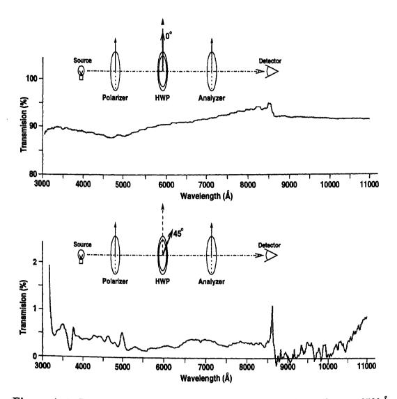
**Figure A.4:** Response curve of the superachromatic HWP The spike at  $\sim 8500$ Å, is an artifact of changeover of detectors.
