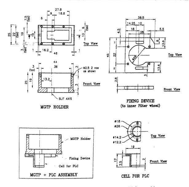
Figure C.7: The analyzer unit: The MGTP + PLC assembly.
