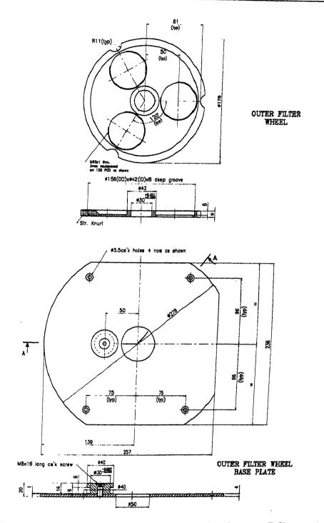
Figure C.6: The online calibration and the second order cutoff filter unit. The "Outer Filter Wheel" and the "Outer Filter Wheel Base Plate".
