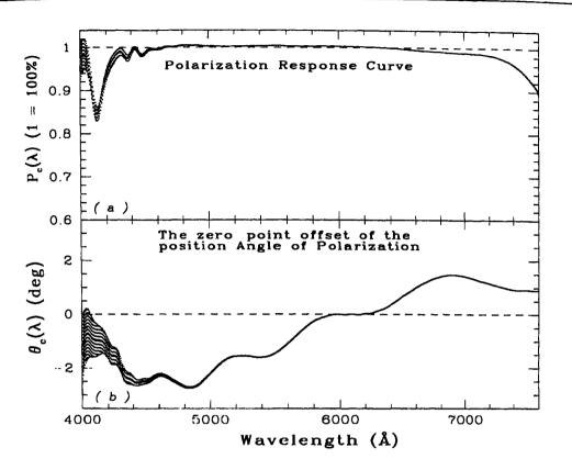
**Figure 3.5:** Variation of the polarization response and the zero point offset of the position angle of polarization with wavelength of the spectropolarimeter.
