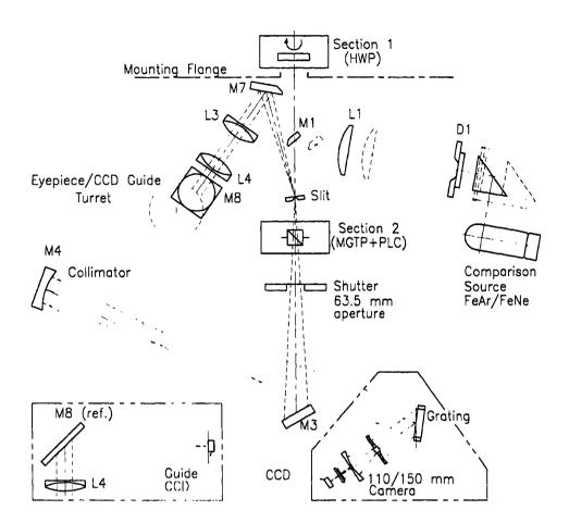
**Figure 3.2:** The optical layout of the Boller & Chivens spectrograph.  $M_3$  is a flat folding mirror. Original drawing Courtesy, Dr. Greg Smith, Mech. & Opt. Design Group, AAO. The drawing has been modified to the present spectropolarimetric set up.
