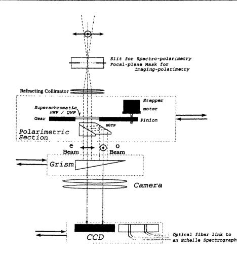
Figure 7.2: A conceptual optical design for the I&S-P (Not to Scale)
