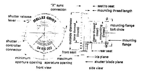
Figure C.9: Shutter for the spectropolarimeter. A 63.5 mm aperture Melles Griot 04 IES 003.
