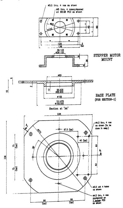
Figure C.4: The stepper motor mount and the base plate for the Section-1
