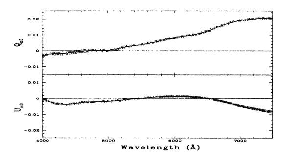
Figure 3.6: Effects of telescope polarization  $Q_{n0}(\lambda)$  and  $U_{n0}(\lambda)$  measured from the observations of unpolarized standards, on 6<sup>th</sup> and 7<sup>th</sup> March 1998. In each case the thick central line is the spline fit to the data. The two enveloping lines are the  $1\sigma$  propagated errors derived from the photon noise errors in the four input spectra  $L_{\alpha}$  (Eqs.3.17 & 3.18).
