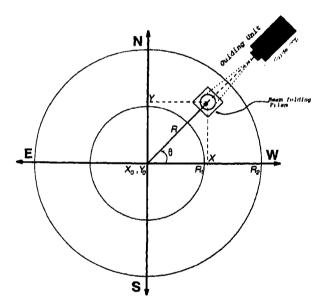
Figure 7.1: Guiding the Telescope with a field star. X increases to the right and  $\alpha$  increases to the left as per convention.
