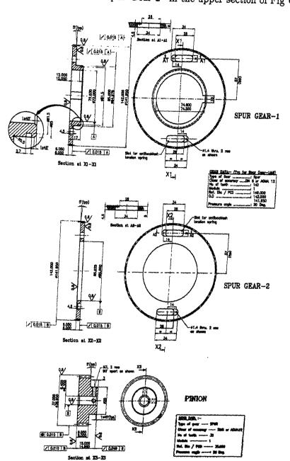
is fixed to a split anti-backlash, on axis spur gear. The split sections of the gear is shown as "Spur Gear 1" and "Spur Gear 2" in the upper section of Fig C.3. The
