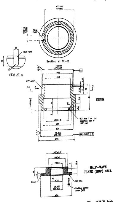
The HWP rotating unit consists of a "HWP holding cell" (Fig C.2, bottom) which holds the Pancharatnam design superachromatic half wave plate (HWP). This cell
