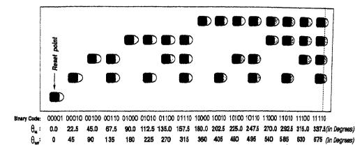
Figure C.5: The outer surface of the mechanical absolute encoder cylinder. The shaded squares are the binary coded grooves. The corresponding binary code along with  $\theta_M$  and  $\theta_{WF}$  (in degrees) are written below. The dotted line near  $\theta_{WF} = 675^{\circ}$ is the joining point to the left end as a completion of the cylinder.
