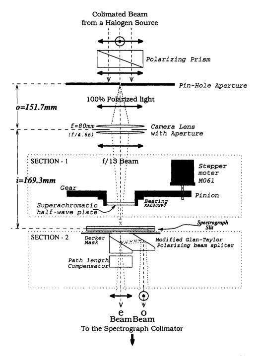
Figure 3.4: The Experimental setup for the calibration with a 100 % polarized source. The polarimetric attachments to the spectrograph, is integrated with Section-1 and Section-2 (Fig. 3.3) (Figure not to Scale).
