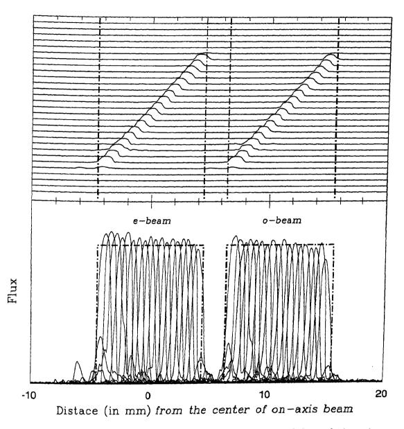
Figure A.8: The scan across the MGTP + PLC. The top panel shows the intensity scans y-shifted to indicate the location of illumination and on the lower panel these are over-plotted for intensity comparison. The vertical dash-dot lines show the limits of the MGTP aperture. The x-axis is centered on the on-axis beam.
