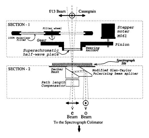
Figure 3.3: Sketch of the two Sections mounted on to the spectrograph to convert it to a spectropolarimeter (Figure not to Scale). Section-1 contains the HWP and Section-2 houses the MGTP + PLC assembly.
