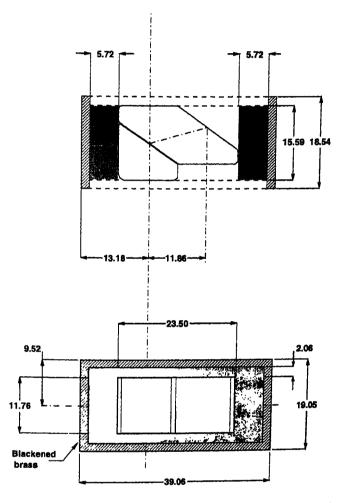
Figure A.5: Drawing of the Modified Glan-Taylor Prism (MGTP) provided by the Karl Lambrecht Corp. (dimensions are in mm).
