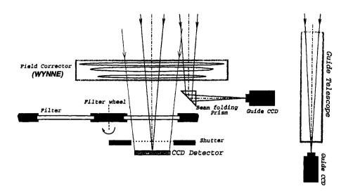
Figure 2.1: Schematic Diagram of the VBT Prime Camera
