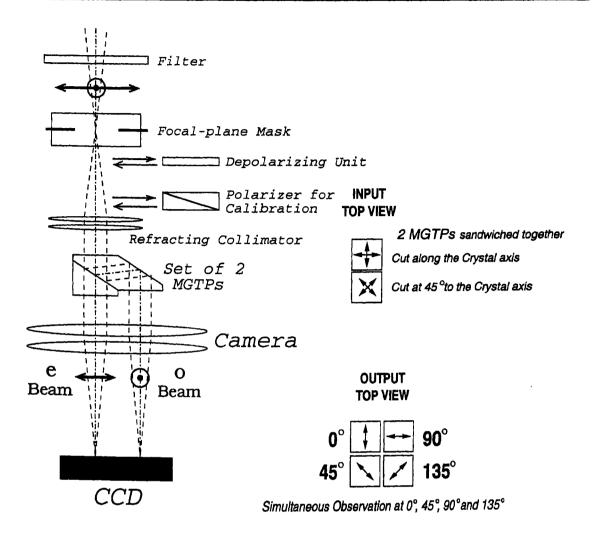
Figure 7.3: A conceptual optical design for the FBImP (Not to Scale)
