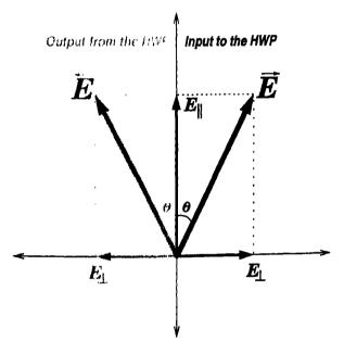
Figure A.2: Input and output wavefronts from a HWP.
