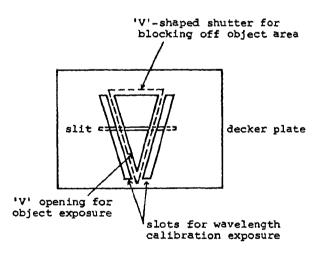
Figure 2.2 Decker plate and slit of the Cassegrain spectrograph used at the F/13 focus of the 102 cm reflector at Vainu Bappu Observatory. outside the arms of the 'V', the latter being covered by a shutter during such exposures (See Figure 2). The slit plane was slightly tilted, so that objects reflected off the slit jaws could be monitored through an eye piece continuously and the telescope guided, during exposures.
