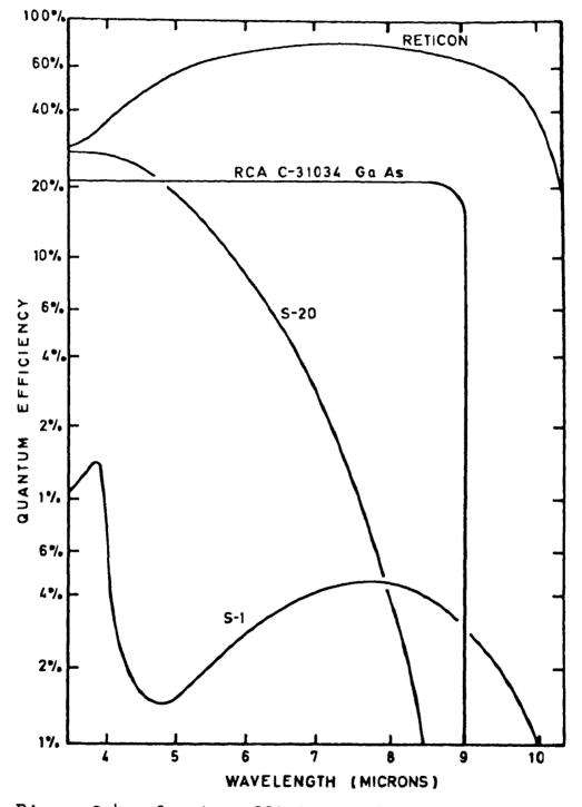
Figure 2.4. Quantum efficiency of the reticon array and several conventional photocathodes
