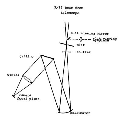
Figure 2.1 Schematic layout of the Cassegrain spectrograph used with the 102 cm telescope F/13 focus at the Vainu Bappu Observatory.
